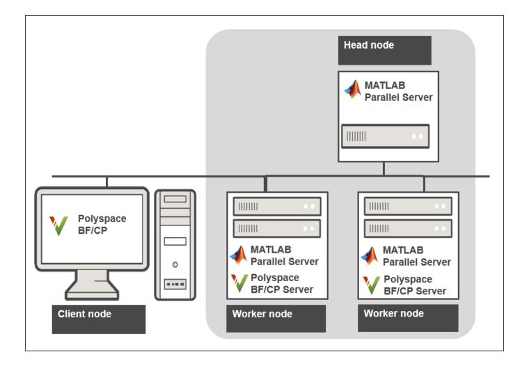
In the simplest remote analysis configuration, the same computer can serve as the head node and worker node. Note that you can run one Polyspace analysis on one worker only. You cannot distribute the analysis over multiple workers. Only if you submit more than one analysis job, you can distribute the jobs over multiple workers.
